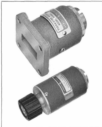
Fig. 7. -hp- 486A waveguide thermistor mount (upper) has been designed in guide sizes from 2.6 to 40 gc. Model 478A coaxial mount (lower) operates from 10 mc to 10 gc.
